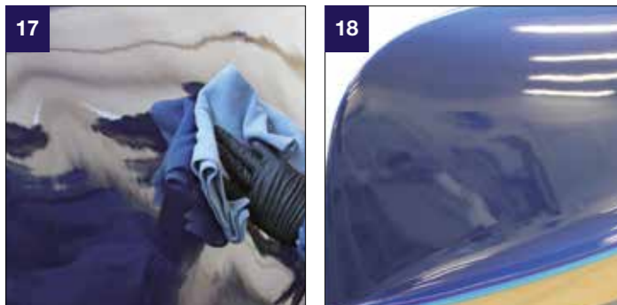
Remove Finish Control Spray with microfibre cloth, check result visually
