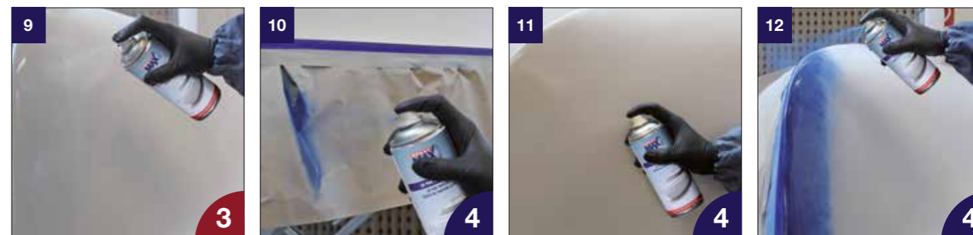
9 Apply 2-4 spray passes, flash off time 5-10 min between each spray pass
