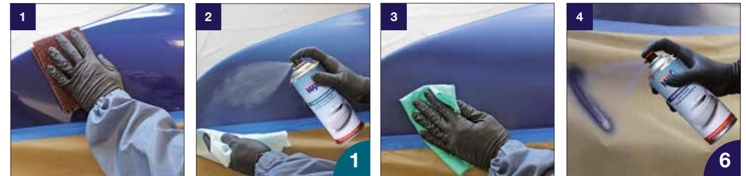
If necessary mask area below water line and sand with abrasive fleece
